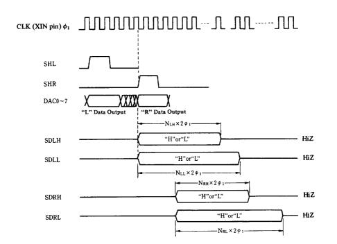
However, NLH, NRL, NRH, and NRL are the number of bits of the absolute value of the difference of the previous sound data. If it is larger than the previous data, the output value is "H", and if it is smaller, the output value is "L"
